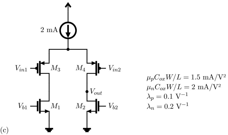
Resposta:  $R_{in} = \infty$ ,  $R_{out} = 3.3 \text{ k}\Omega$ ,  $A_{v0} = -2.9 \text{ V/V}$ .
