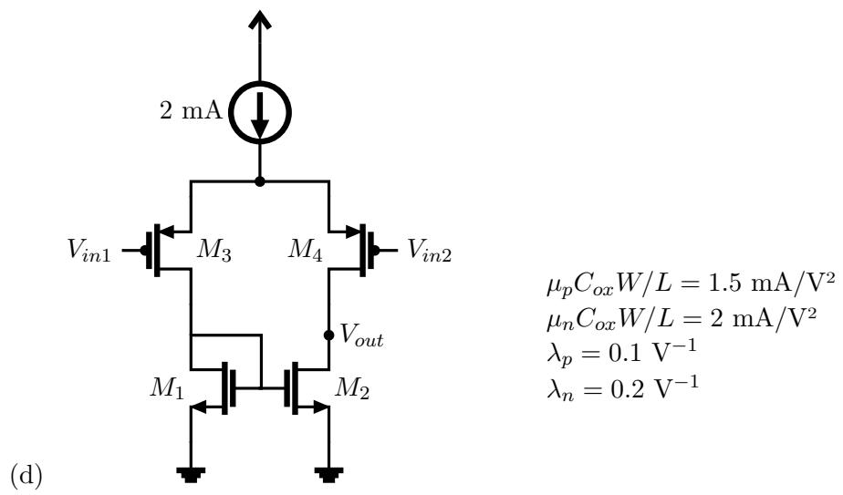
Resposta:  $R_{in} = \infty$ ,  $R_{out} = 3.3 \text{ k}\Omega$ ,  $A_{v0} = 5.8 \text{ V/V}$ .
