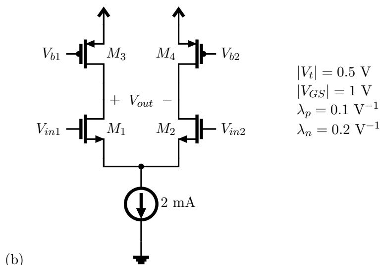
Resposta:  $R_{in} = \infty$ ,  $R_{out} = 6.7 \text{ k}\Omega$ ,  $A_{v0} = -13.3 \text{ V/V}$ .
