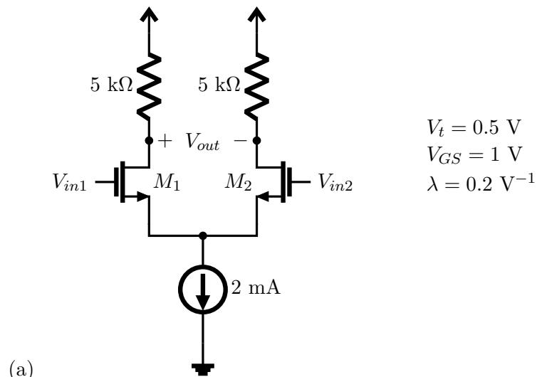
Resposta:  $R_{in} = \infty$ ,  $R_{out} = 5 \text{ k}\Omega$ ,  $A_{v0} = -10 \text{ V/V}$ .
