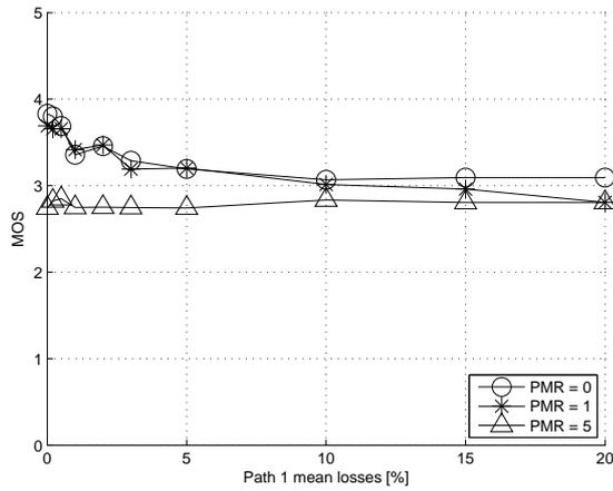
Fig. 4. Path 0: delay = 30ms and losses = 3%. Path 1: delay = 10ms.
