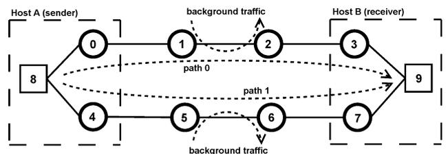
Fig. 2. Topology used in all simulations. Each link is full-duplex, with transmission rate of 1Mbps and 30ms of propagation delay. Background traffic between nodes 1 - 2 (path 0) and 5 - 6 (path 1). Losses occur in the links between nodes 2 - 3 and 6 - 7. Path 0 is set to primary at the beginning of each simulation.
