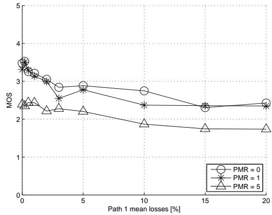
Fig. 6. Path 0: delay = 10ms and losses = 15%. Path 1: delay = 30ms.
