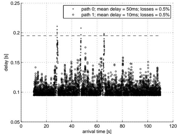
Fig. 3. Results from a single simulation. Circles are packets that arrived from path 0. Crosses are packets that arrived from path 1. X axis is the packet arrival time and Y axis is its delay. The dashed line is the jitter-buffer threshold. In this simulation, PMR = 1 and delay-centric algorithm is active.
